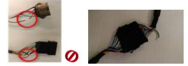
5 - Disconnect the connections to check the condition of the pins and reposition them if they are bent
