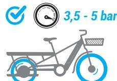
2. In order to improve battery life and efficiency, pump the tyres to between 3.5 and 5 bar
