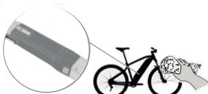
All cleaning work must be done with the battery on the bike but the bike turned off! That way, the battery connections will be hidden and protected from the water.
