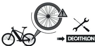
The motorised wheel is also subject to higher stress than a standard bike wheel, and although it is reinforced, it is possible that spokes may break. If a spoke breaks, contact your DECATHLON store.
