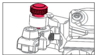
TRP does not recommend the use of inline barrel adjusters. These are for use on mechanical brakes to compensate for pad wear. Using inline barrel adjusters will increase the risk of accidentally riding with a closed system.
