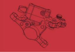
The HYRD brake system is an open hydraulic brake designed for use on single rider bicycles. The purpose of the open hydraulic system is to allow the pistons to compensate for pad wear. Each time the brake is released, the piston opens up the reservoir, allowing more oil into the caliper if needed. Only a properly set-up brake will allow the piston to retract fully ensuring that your brakes can account for worn pads.
