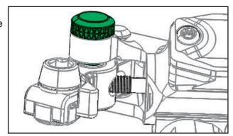
If the Lock Knob will **NOT** thread into the actuator arm or is very difficult, this means that the actuator arm is preventing the piston from returning fully and has closed off the reservoir port. This prevents the brake to compensate for pad wear.
