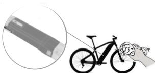
All cleaning work must be done with the battery on the bike but the bike turned off! That way, the battery connections will be hidden and protected from the water.
