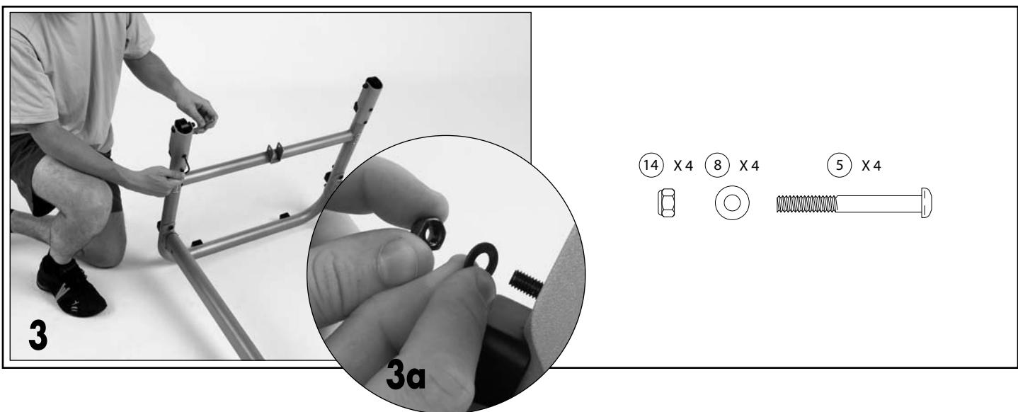
MONTAGE • ASSEMBLY • MONTAJE • MONTAGE • MONTAGGIO • AFWERKING
