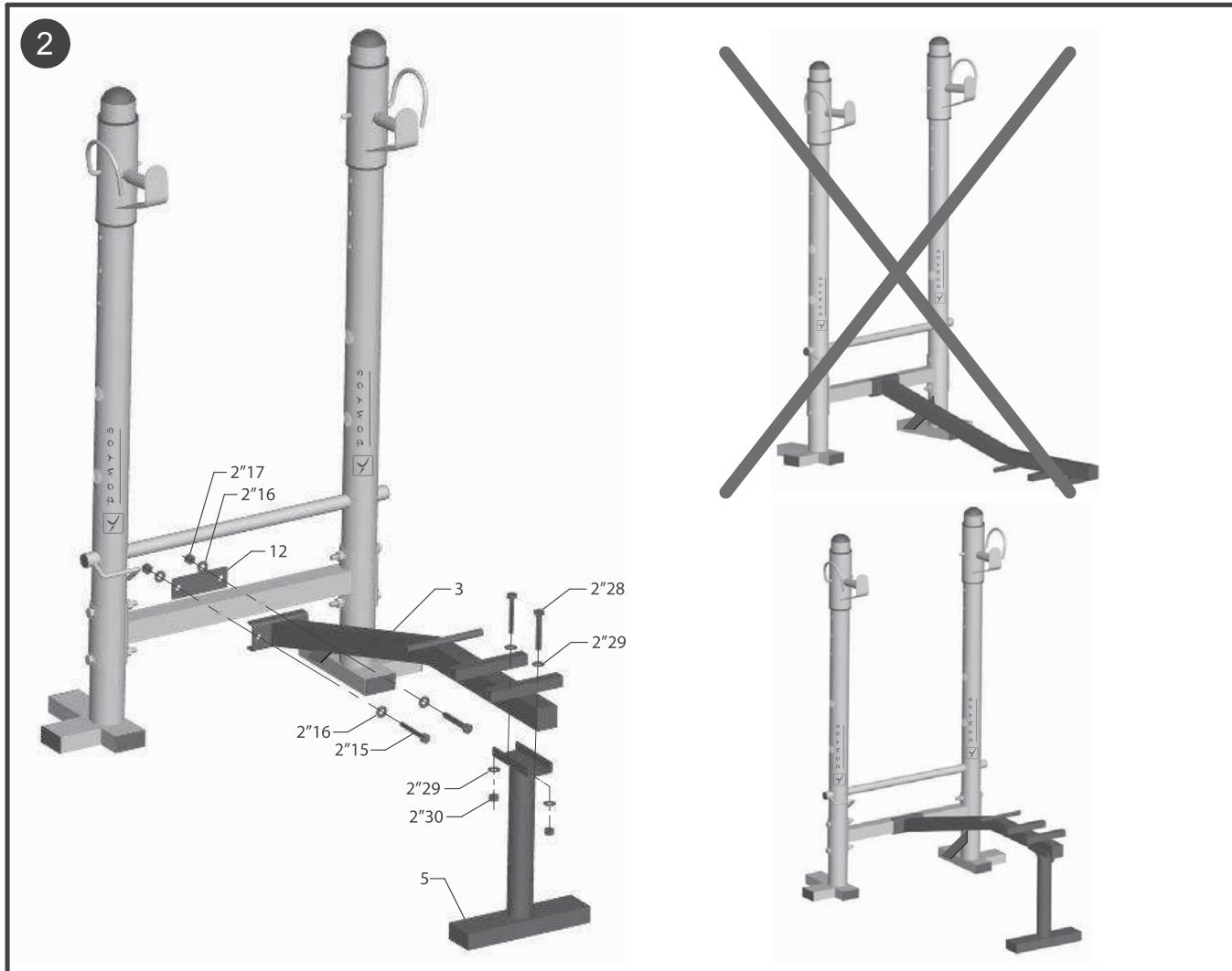
**ASSEMBLY • MONTAGE • MONTAJE • MONTAGE • MONTAGGIO • AFWERKING
