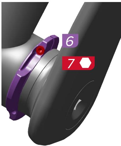
To preload the crankset, turn the preload adjuster in the direction of the + sign until it stops. Tighten the preload adjuster bolt to close the gap. Check the crankset for play by rocking the crank arms back and forth.
