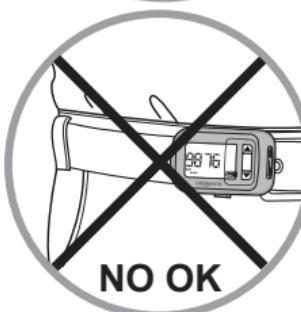
This pedometer is designed to measure the different parameters of your steps on flat ground. Technically, these measurements are taken by recording shock waves caused when your foot makes contact with the ground; this requires the product to be attached somewhere around the hip (trouser or shorts belt).
