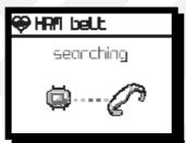
To detect the signal from the belt, it must be fitted to the chest with the sensors moistened. If after several attempts the belt cannot be recognised, try pairing using this mode.
